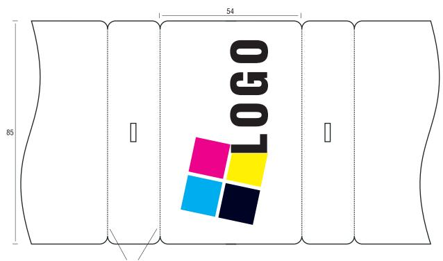
Micro perforation to the separating edges allows the simple and clean extraction of the cards from the label web.
